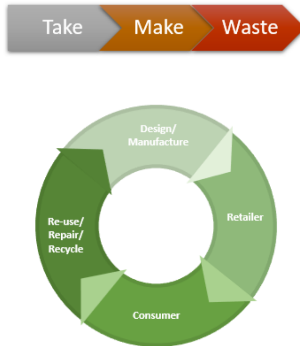
Figure 2: Diagram to illustrate the difference between (top) a traditional, 'linear' economy, in which raw materials are extracted from the environment, used in manufacturing, and then disposed of; and (bottom) a 'circular' economy, in which materials are kept in use for as long as possible by reusing or recycling products at their end-of-life.
